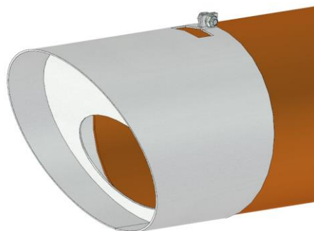
c) Clamped to the spigot end of the pipe
